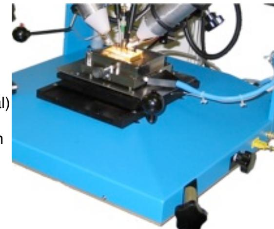
**GAS NOZZLES:** our standard quartz-glass nozzles range from .02" - .24" orifice size, and come angled (to blow directly down) and straight. For special applications we can make rectangular shapes, with or without baffles, and custom shapes as well. Nozzles changes take 1-2 minutes.
