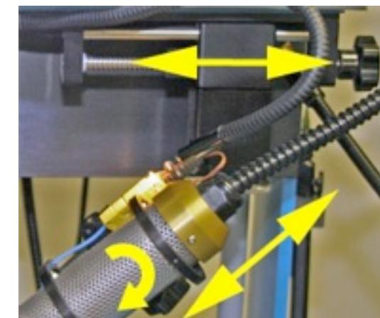
**JET POSITIONING:** Each heater jet is mounted on a swing-out arm with horizontal (leadscrew) and vertical (rack & pinion) positioning with adjustable stops, and each can be rotated to access corners and clear package features. Angled nozzles can also be rotated in their holders to provide additional coverage options. Operators can easily align nozzles with the target die, and bring them as close as necessary to control overflow.
